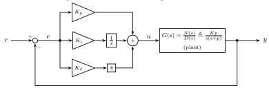
(i) The r-to-y and r-to-u transfer functions are:
